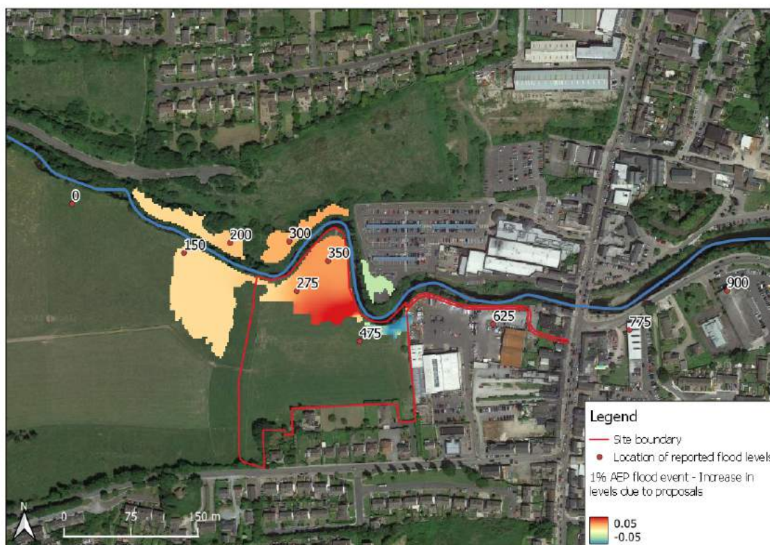
Figure 32: Changes in flood levels due to proposals 1% AEP (red shows increase, blue decrease)
