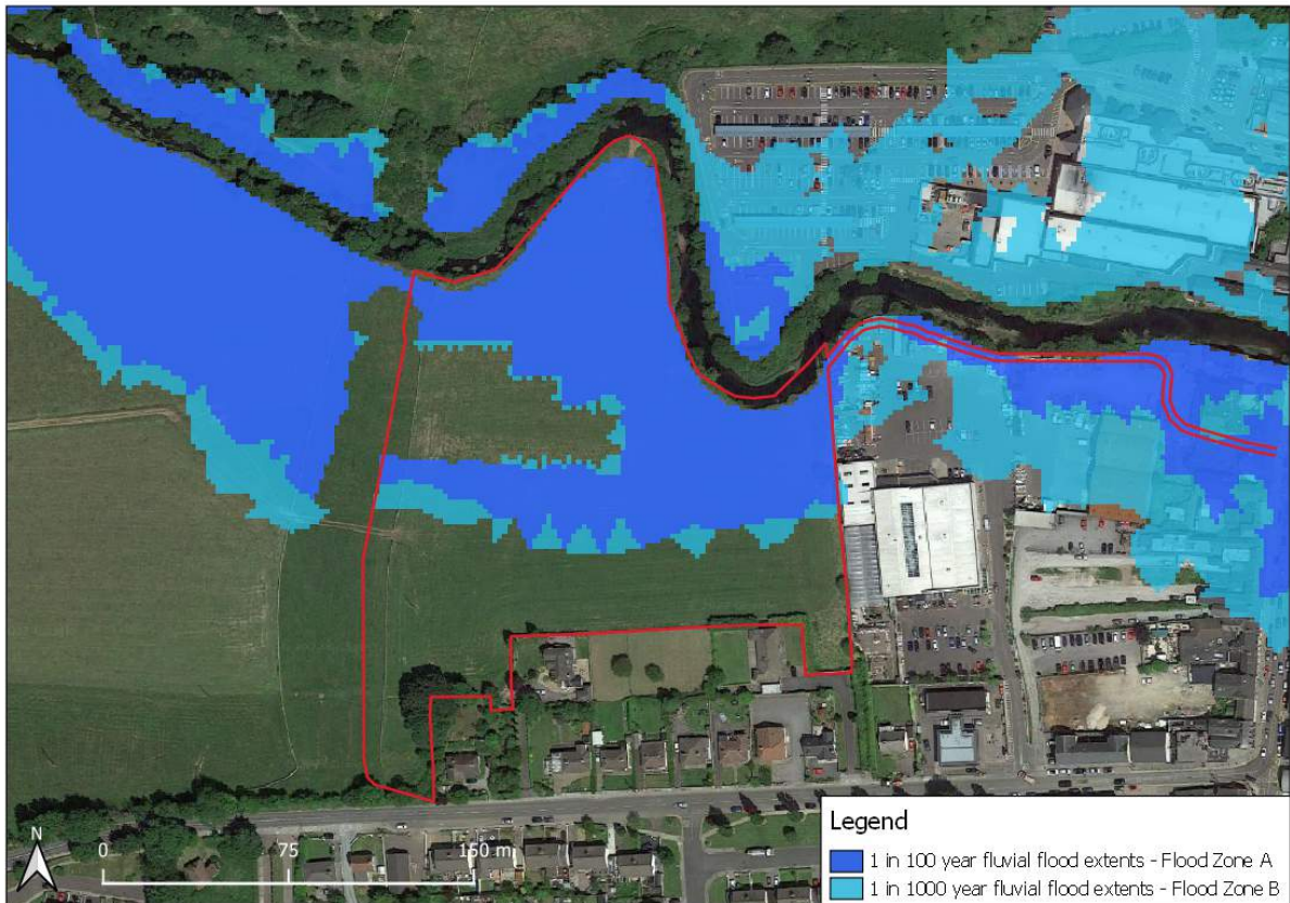
Figure 26: Arup model Baseline fluvial flood extents. 1% AEP (1 in 100 year) and 0.1% AEP (1 in 1000 year) events (Flood Zones A and B)
