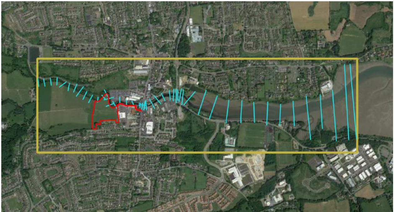
Figure 20: Cross-section location of river channel survey
