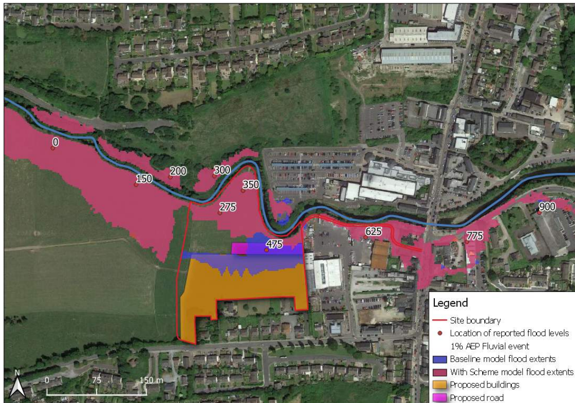
Figure 31: Flood extents during Baseline and With Development scenarios (1%AEP fluvial flood event)
